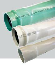
DURALOC® pipe is manufactured using a high-strength, high-impact PVC compound, providing enhanced protection against cracking, leaking, corrosion, and other threats to ensure long-lasting infrastructure. Resistant to H<sub>2</sub>S and other aggressive chemicals commonly found in sanitary sewage, this pipe maintains its integrity over time. With a Manning coefficient of 0.009, it allows for the use of smaller diameters compared to other materials, without compromising performance.
